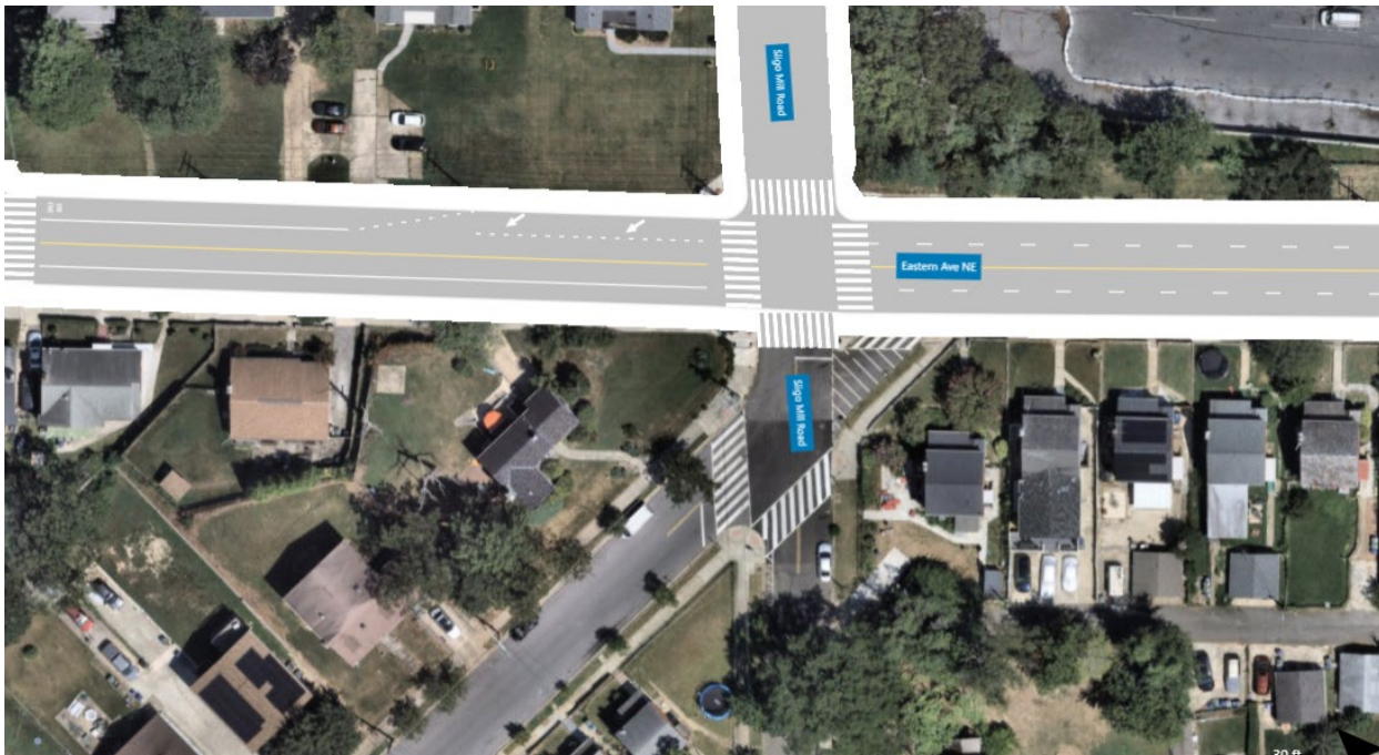
Figure 3: Proposed safety treatment at Sligo Mill Road and Eastern Ave NE intersection
